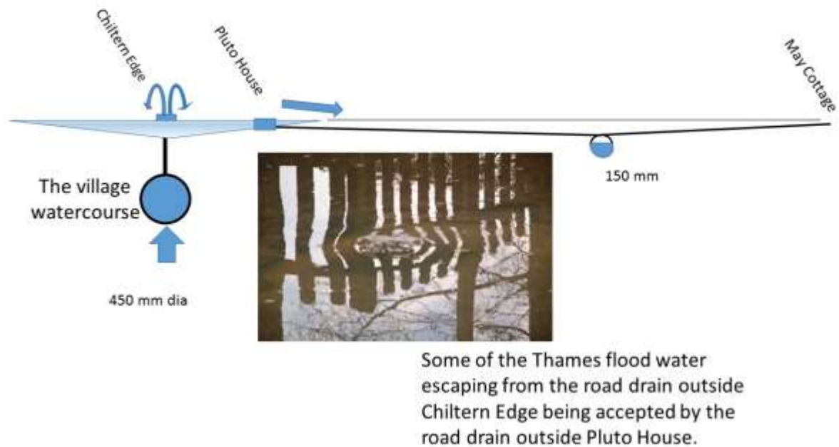
Figure 5 - Schematic of the two road drain systems in Eastfield Lane, looking north
